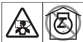
The Engine emits toxic Carbon Monoxide. Do not run the Engine in an enclosed area.
