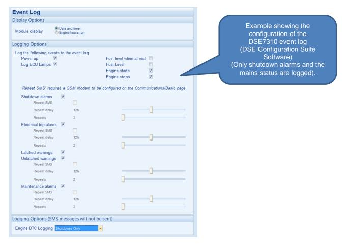
Once the log is full, any subsequent shutdown alarms will overwrite the oldest entry in the log. Hence, the log will always contain the most recent shutdown alarms.
