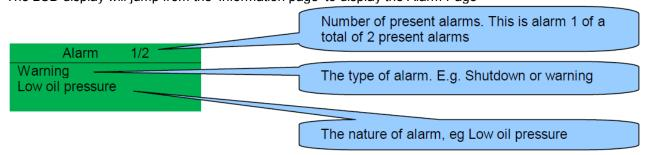
The LCD will display multiple alarms E.g. "High Engine Temperature shutdown", "Emergency Stop" and "Low Coolant Warning". These will automatically scroll in the order that they occurred.
