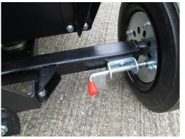
5.2.3 Place pin through turnbuckle and tighten
